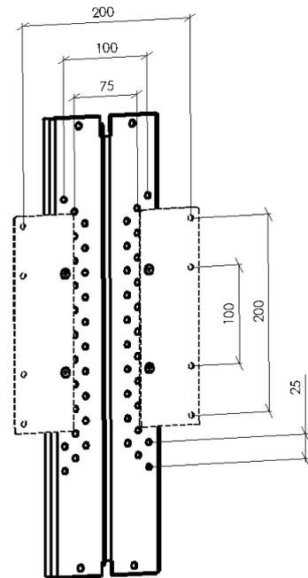
Plasma/LCD mounting bracket for use with TS460.
