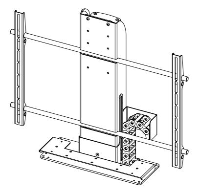
Smooth, whisper quiet, screen lifting mechanism with 675mm of travel
